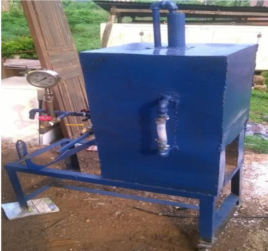
Figure 5: Picture of the developed miniature steam boiler for the generation of steam
