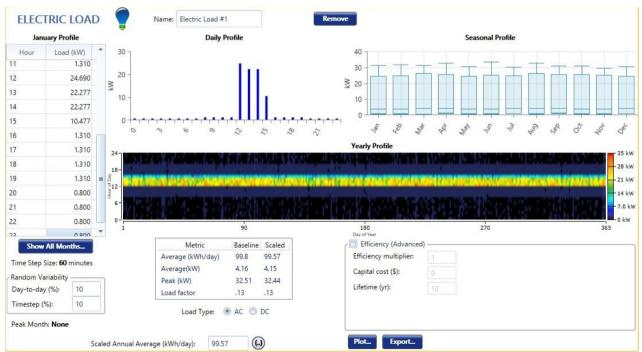
Figure 3: Load profile with 10% allowance
