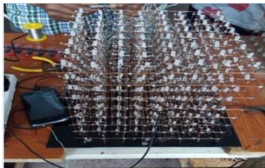
Figure 9 Completely formed 8 \times 8 \times 8 LED cube array
