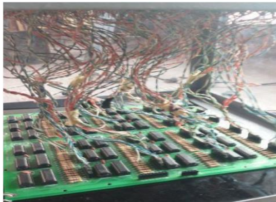
Figure 20 Cathode driver with mounter ICs and wires connected to the LED cube
