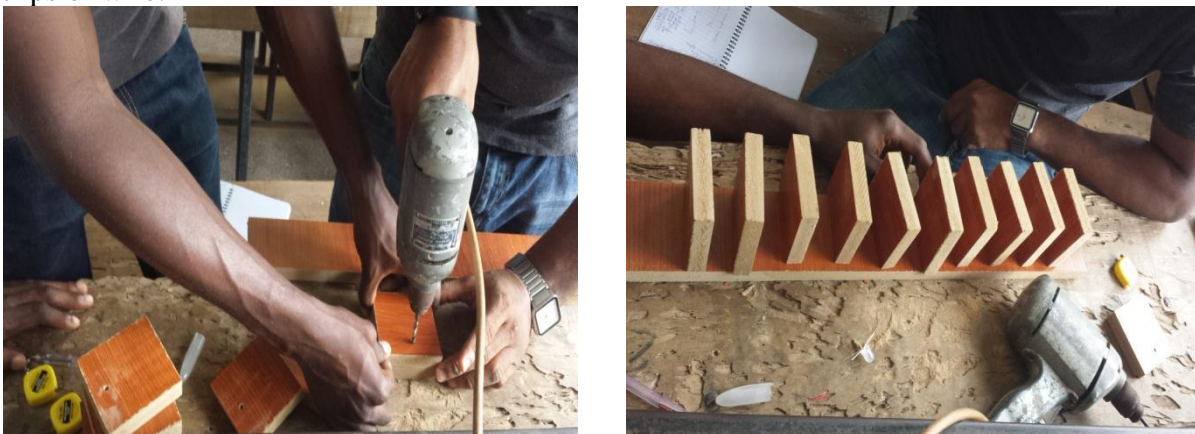
Figure 3 Forming the jig
