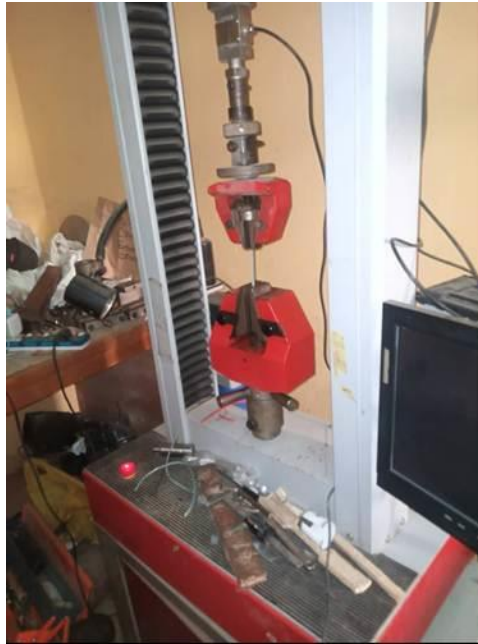
Figure 1: A composite sample undergoing tensile strength testing
