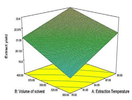
Figure 2: Three-dimensional plots showing the effect of volume of solvent and extraction temperature on the extract yield
