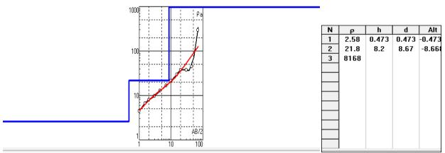
Figure 16. The Sounding curve and interpretation model for VES05 along Profile 3
