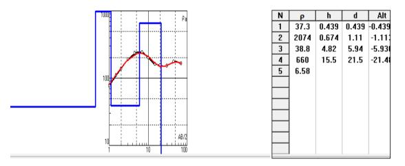
Figure 13. The Sounding curve and interpretation model for VES02 along Profile 3
