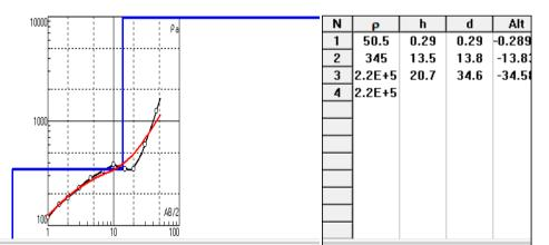
Figure 6. The Sounding curve and interpretation model for VES04 along Profile 1
