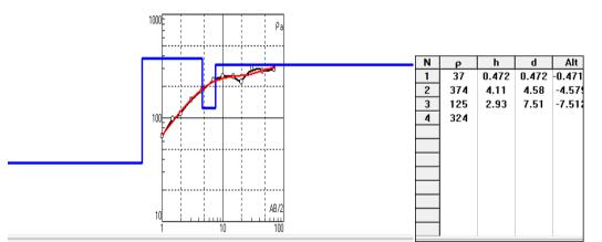
Figure 15. The Sounding curve and interpretation model for VES04 along Profile 3
