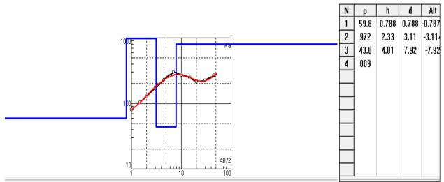
Figure 9. The Sounding curve and interpretation model for VES02 along Profile 2
