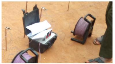
Plate 1 Terrameter, wire cables and reel
