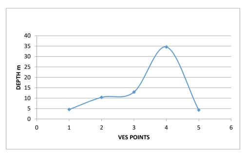
Figure 17. Basement Topography along Profile 1
