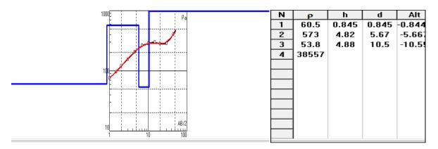
Figure 11. The Sounding curve and interpretation model for VES05 along Profile 2
