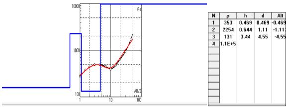
Figure 3. The Sounding curve and interpretation model for VES01 along Profile 1.
