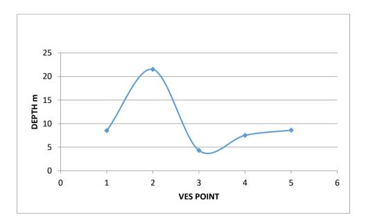
Figure 19. Basement Topography along Profile 3
