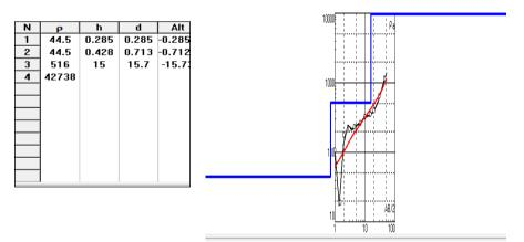
Figure 8. The Sounding curve and interpretation model for VES01 along Profile 2
