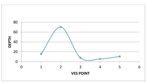
Figure 18. Basement Topography along Profile 2
