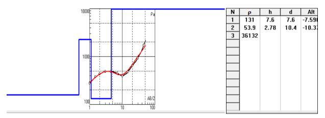
Figure 4. The Sounding curve and interpretation model for VES02 along Profile 1
