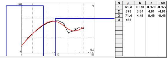
Figure 12. The Sounding curve and interpretation model for VES01 along Profile 3
