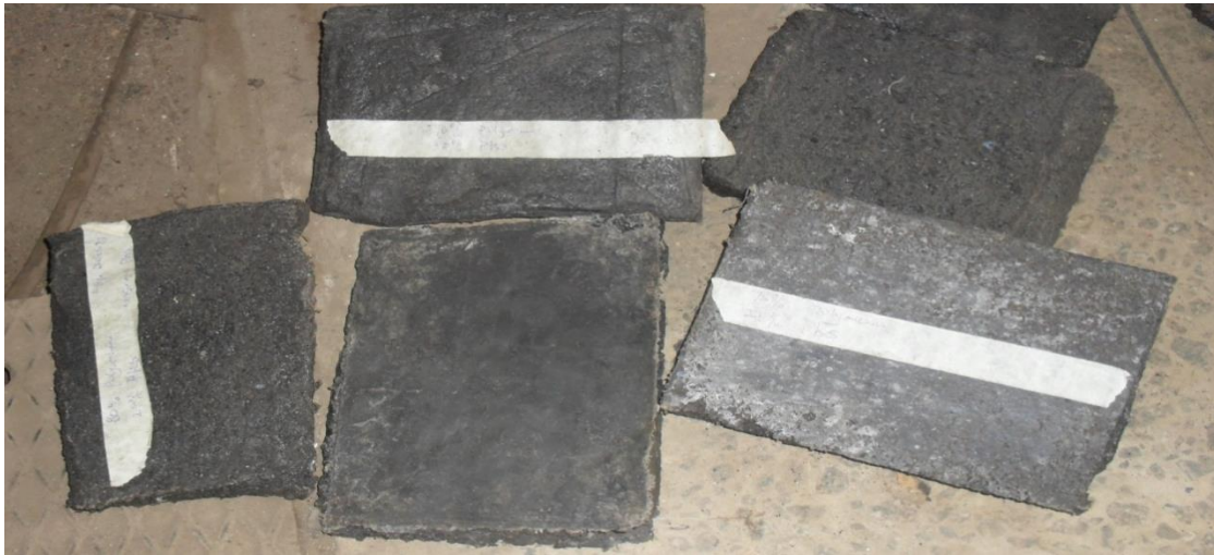
Fig. 2: Composite materials of the different compositions after ejection from mould
