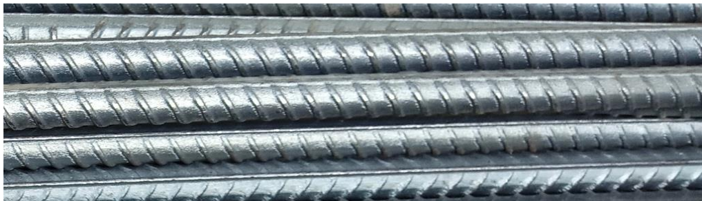
Figure 2: Rib pattern of some of the studied TMT reinforcements in Nigeria
