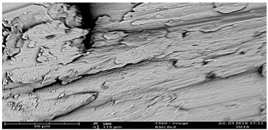
Plate 3. Fracture Surface of Test Specimen of Medium Heat Inputs at 500X Magnifications
