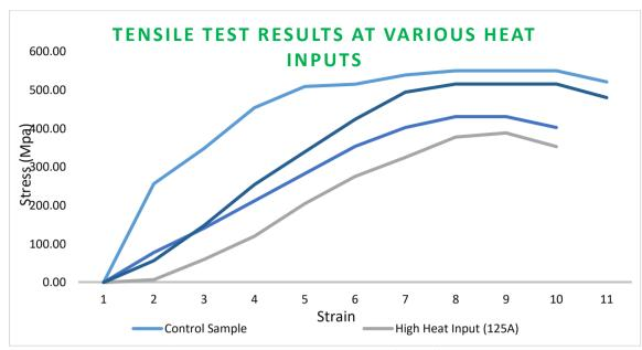
Figure 2. Tensile Test Results of the Samples
