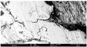
Plate 2. Fracture Surface of the Test Specimen of Low Heat Input at 500X Magnifications
