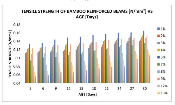
Figure 4: A graph of Tensile strength of Bamboo Reinforced Beams versus Age
