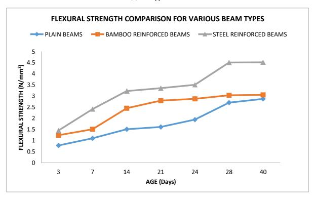
**Figure 6:** A graph of flexural strength comparison for plain beams, Bamboo- reinforced beams and steel-reinforced beams
