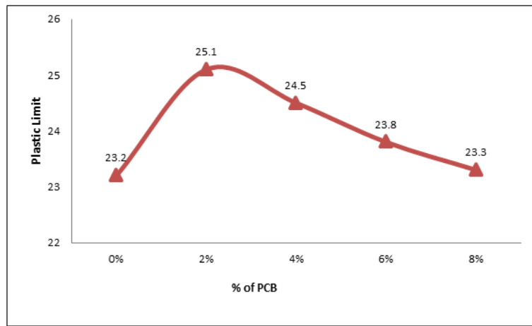
Figure 4. Plastic Limit results for the Lateritic soil with mix proportions of PCB
