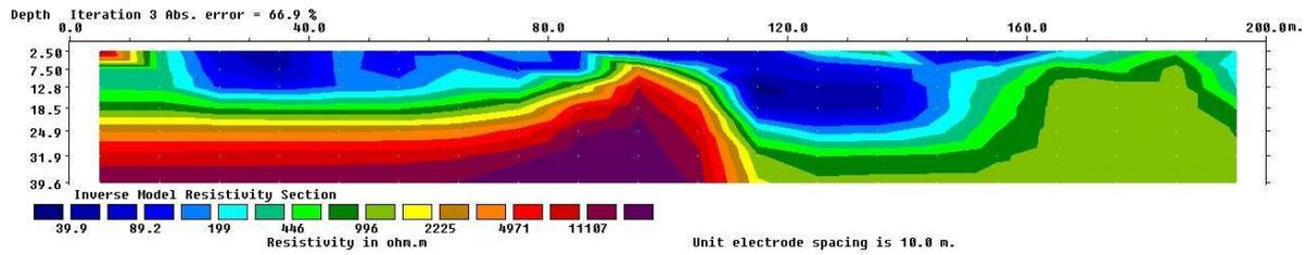
Figure 7: The inverse model resistivity section for Traverse 5.
