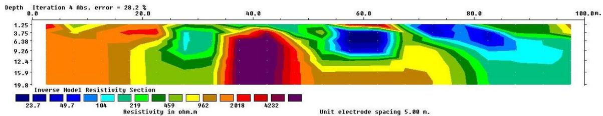
Figure 8: The inverse model resistivity section for Traverse 6
