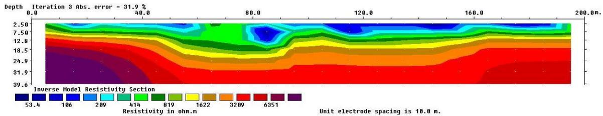
Figure 3: The inverse model resistivity section for Traverse 1
