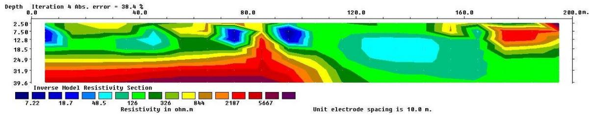
Figure 6: The inverse model resistivity section for Traverse 4.
