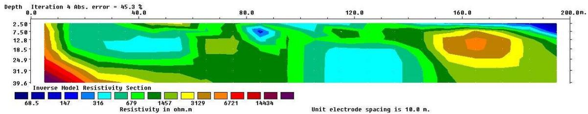
Figure 4: The inverse model resistivity section for Traverse 2
