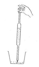
Figure 3: Transfer of liquid in pipette to a container. Source [3]
