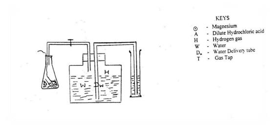
**Figure 1:** Apparatus for determination of volume of hydrogen produced in a reaction between magnesium and hydrochloric acid. Source [2]
