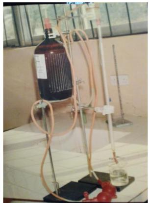
**Figure 6:** *The photograph of the designed positive pressure dispenser*
