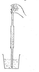
Figure 2: Use of pipette to lift liquid. Source [2]
