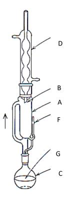
Figure 4: Soxhlet apparatus. Source [4]
