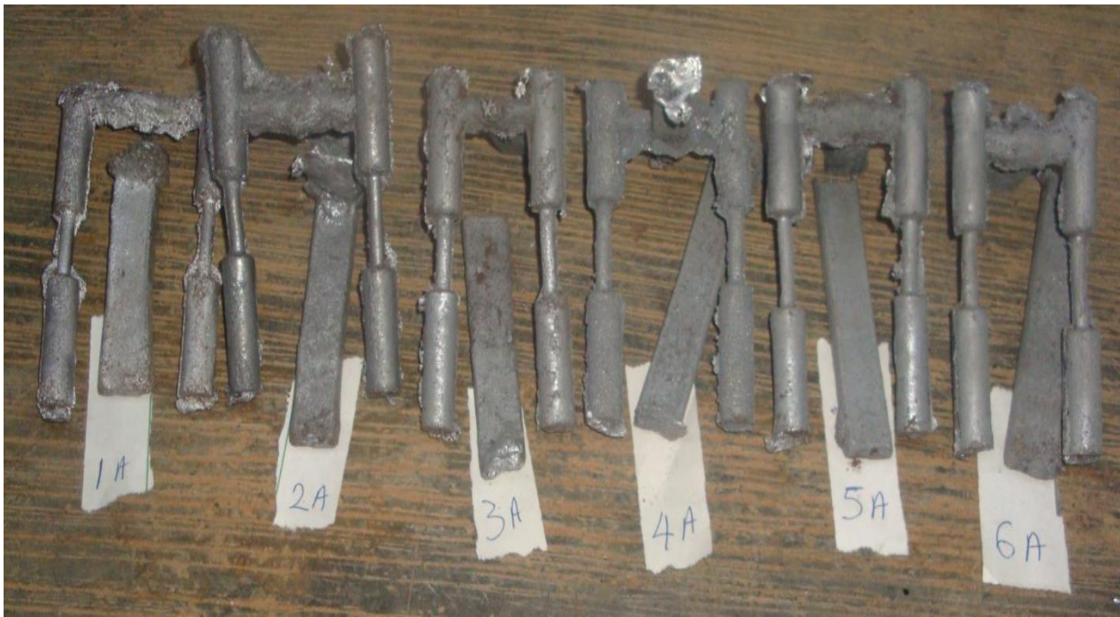
Figure 1. Photograph of the cast Pb-Sb-Zn alloys
