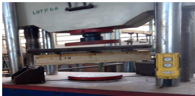
Figure 2: Box Specimen loaded on the Digital Board Universal testing machine
