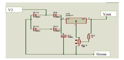
Figure 3. Bridge rectifier and Voltage regulator circuit diagram
