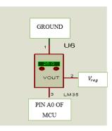
Figure 5. LM35 Temperature Sensor
