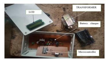
Figure 10. Battery Charger under construction
