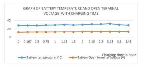
Figure 12. Graph of the battery voltage level and temperature with respect to time
