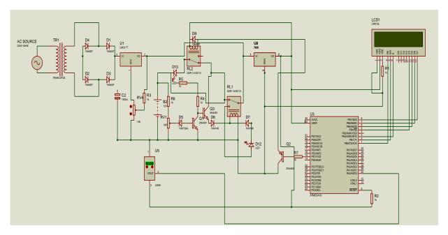
Figure 9. Circuit diagram of the Automatic temperature control lithium-ion battery charger
