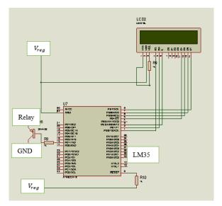
Figure 6. ATMEGA 328P Microcontroller and Liquid Crystal Display
