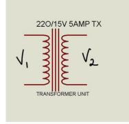
Figure 2. Schematic diagram of a 220/15V stepdown transformer.
