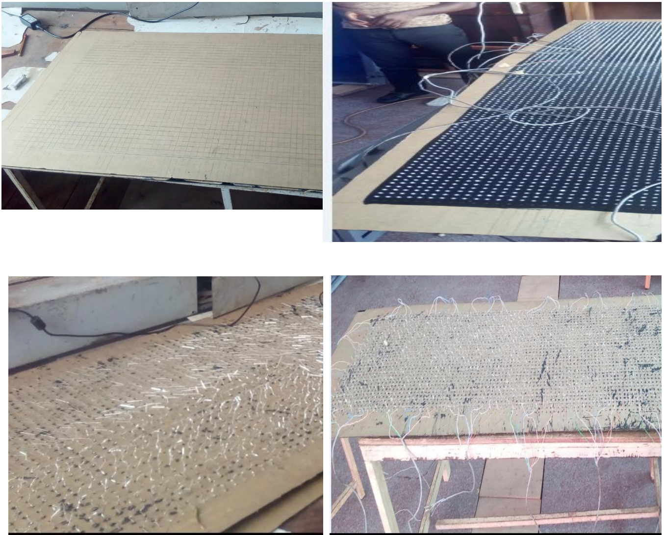
Figure 3 (a) Marked Perspex board (b) LED matrix board with LED (c) twisting of LED on the board the circuit and (d) LED board with soldered connectors
