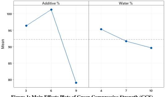
Figure 1: Main Effects Plots of Green Compressive Strength (GCS)
