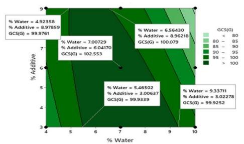
Figure 4: Contour plots of a Response (GCS) vs. % Additive and % Water Content
