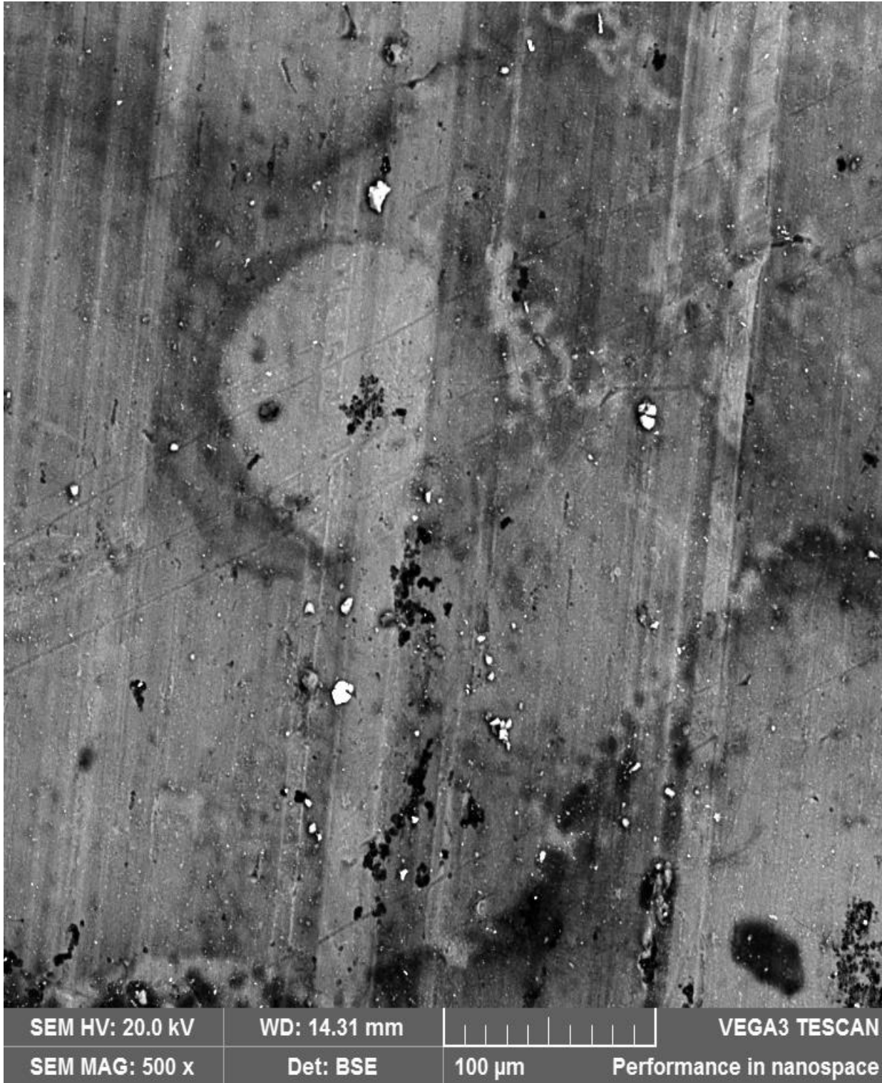
Figure 13: Wear worn surface of the epoxy-5wt% Palm kernel ash nanoparticles
