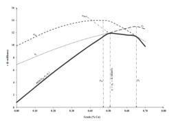
Figure 2 Choosing the Optimum Cut-off in Lane's Model, Source: [20]
