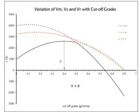
Figure 3 Choosing Optimum Cut-off Grade for Year 1 (Initial Iteration, V=0)
