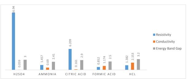
Figure:4: Plot of different dopants showing the level of resistivity, Conductivity and Energy band gap
