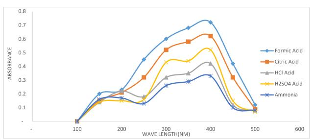
Figure 1: Variation of absorbance with wavelength for different doped poly-aniline material
