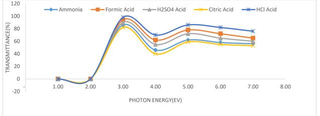
Figure 3: Variation of transmittance with photon energy for doped polyaniline materials.
