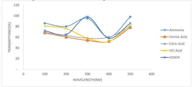
Figure 2: Variation of transmittance with wavelength for different doped polyaniline materials
