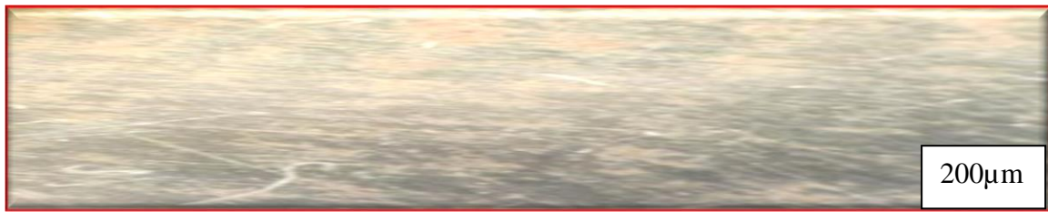
Plate X: SEM surface morphology of a sample from the failure location after it was immersed continuously for 1200 hours in as-received gasoline media
