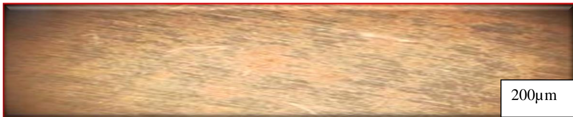
Plate XI: SEM surface morphology of a sample from the failure location after it was immersed continuously for 1200 hours in the as-received diesel media
