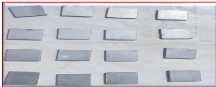
Plate VII: Some of the polished coupons
