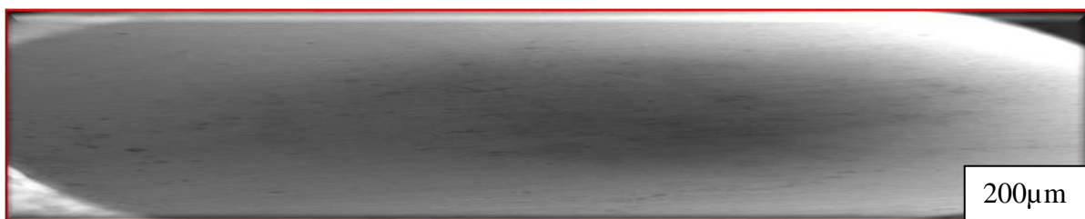
Plate XIII: SEM surface morphology of sample from steel got on the semi-trailer shell adjacent the shell failure location after it was immersed continuously for 1200 hours in the as-received diesel media
