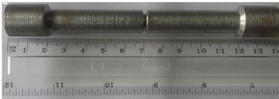
Figure 2: A picture of the notched specimen used for this research
