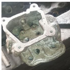
Figure 2a: The plan view of the cylinder head
