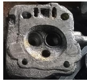
Figure 2b: The bottom view of the cylinder head
