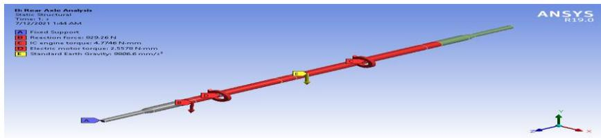
Figure 10: Constraints and loading for rear shaft analysis
