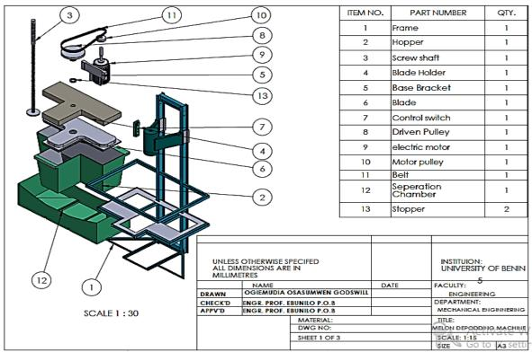
Figure 5. Exploded view of labelled melon depodding machine To design for the power required to operate the machine, Equation 5 can be employed [21].
