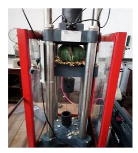
Figure 2a. Melon Pod during cutting test
