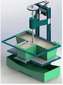
a. orthographic view of melon depodding machine b. Isometric view of melon depodding machine Figure 4. Orthographic and isometric view of melon depodding machine
