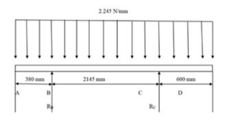
Figure 2: Load distribution on the chassis
