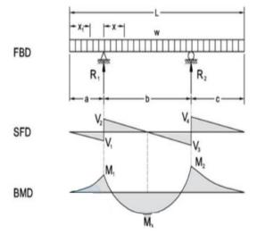
Figure 4: Shear force and bending moment diagram
