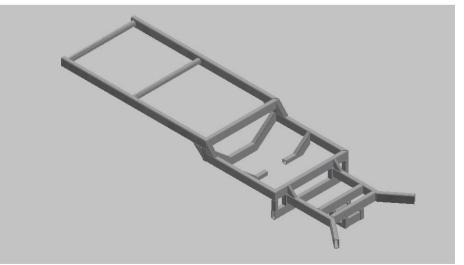
Figure 1: CAD model of chassis in Autodesk Inventor
