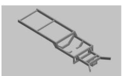
Figure 6: CAD model of chassis in Autodesk Inventor
