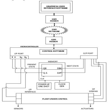
Figure 2: Block Diagram of the Developed System
