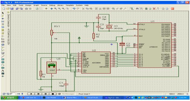
Figure 4: Interfacing the temperature sensor Lm35 to the microcontroller AT89C51
