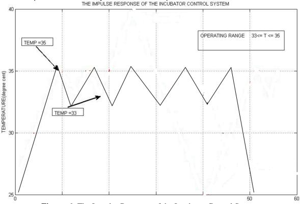
Figure. 6: The Impulse Response of the Incubator Control System
