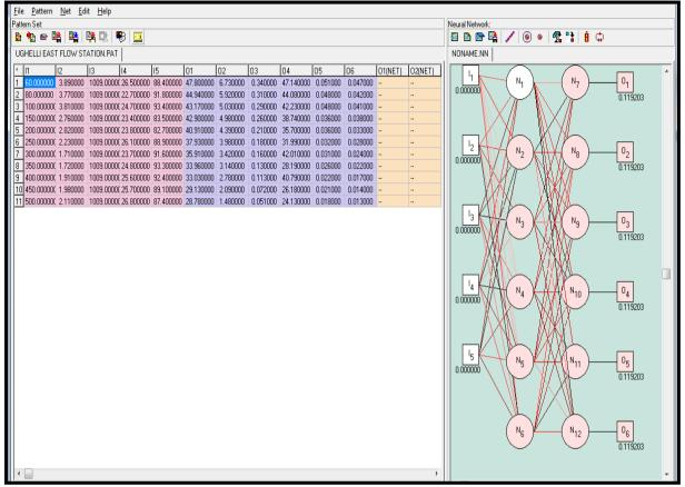
Using the network of Table 5, the Repro Pattern Set function of the Pythia program was then activated to predict the pollutants concentrations based on the input and output data from Ughelli East flow stations. Reliability plots of the field data and the ANN predicted data were obtained to test the correlation between the field data and the ANN predicted data.
