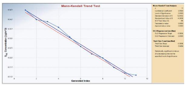
Figure 8: Mann-Kendall Trend Test of SO2 Data from Ughelli East Flow Station
