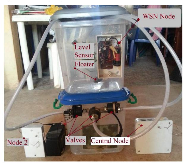
Figure 4. Prototype showing a central node, 2 remote nodes and 3 valves
