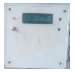
Figure 5. Central node with state of three valves (T1-T3) displayed on LCD
