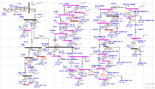
Figure 3: Load Flow Diagram of the Enhanced Iyowa 11/0.415 kV Distribution Network
