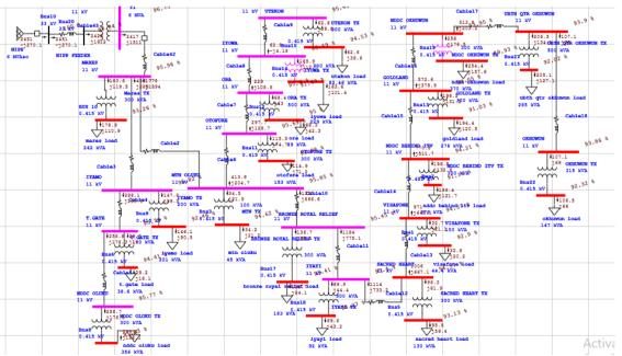
Figure 2: Load Flow Diagram of Iyowa 11/0.415 kV Distribution Network
