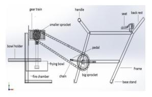
Figure 4: Side View of the Pedal Operated Garri Frying Machine
