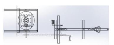
Figure 2: Plan View of Pedal Operated Garri Frying Mach
