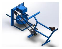
Figure 5: Rendered Isometric View of the Pedal Operated Garri Frying Machine
