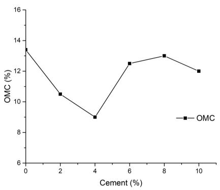
Figure 2: Effect of cement addition on the OMC of the natural soil
