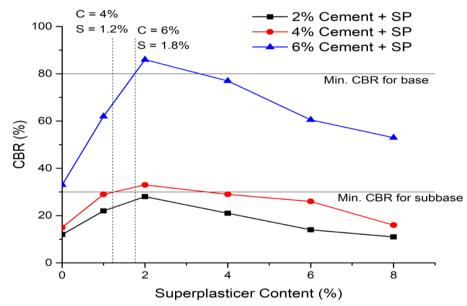
Figure 7: Effect of cement and superplasticiser addition on the CBR of the natural soil
