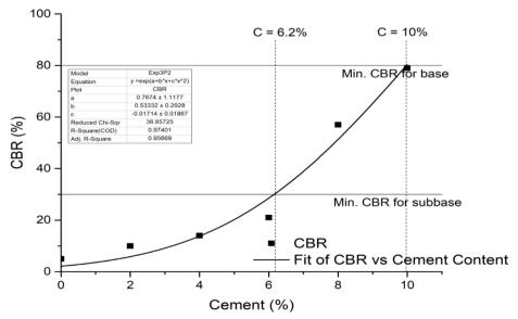
Figure 4: Impact of cement addition on the CBR of the natural soil
