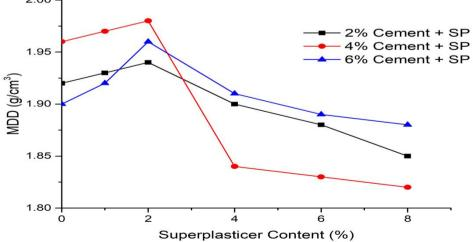
Figure 6: Effect of cement and superplasticiser addition on the MDD of the natural soil
