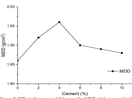
Figure 3: Effect of cement addition on the MDD of the natural soil
