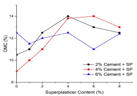
Figure 5: Effect of cement and superplasticiser addition on the OMC of the natural soil
