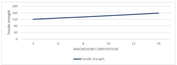
Figure 3. Increasing Tensile Stress with Increase in Magnesium Composition
