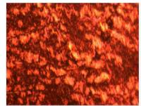
Figure 4. Micrograph of Al-Mg alloy with 14% wt composition of magnesium with 100% magnification
