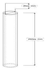
Figure 1. Pattern used for creating the mold
