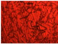
Figure 3. Micrograph of Al-Mg alloy with 8% wt composition of magnesium with 100% magnification
