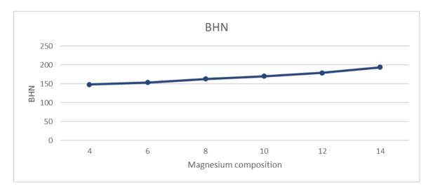
Figure 3. Increasing Hardness with increasing Magnesium Concentration
