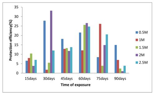
Figure 4: Variation of protection efficiency with exposure time
