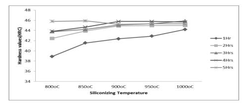
Figure 1: Variation of hardness values with siliconizing temperatures
