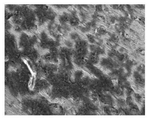
Plate 2: SEM corroded surface of the siliconized samples after 90days in 2.5MHCl at1000X Magnification
