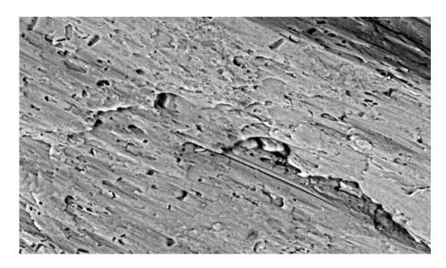
Plate 1: SEM corroded surface of the unsiliconized samples after 90days in 2.5MHCl at 1000X
