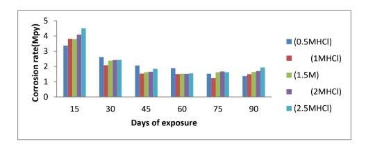
Figure 3: Variation of corrosion rate with exposure time for the siliconized sample
