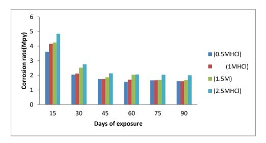
Figure 2: Variation of corrosion rate with exposure time for the unsiliconized sample
