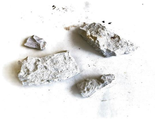
Figure 3. Disintegrated pica at a firing temperature of 300 °C.
