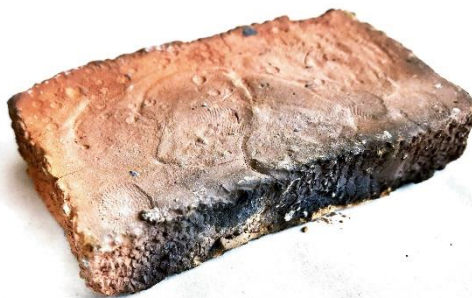
Figure 5. Anthill after firing at 1400 °C – 1550 °C for 1 h
