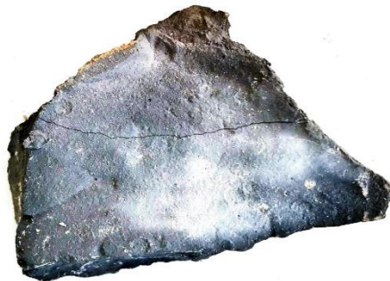
Figure 4. 50% blend ratio of pica and anthill brick after firing at 800 °C to 900 °C for 1 h.
