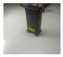
Figure 5: Recycled laptop power pack fitted with tyres
