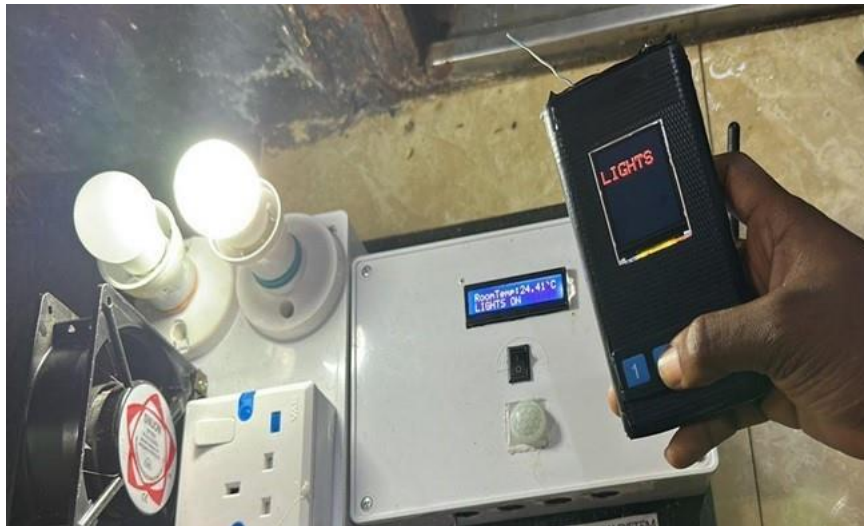
Figure 4: Completed design of the smart home automation system in ON state
