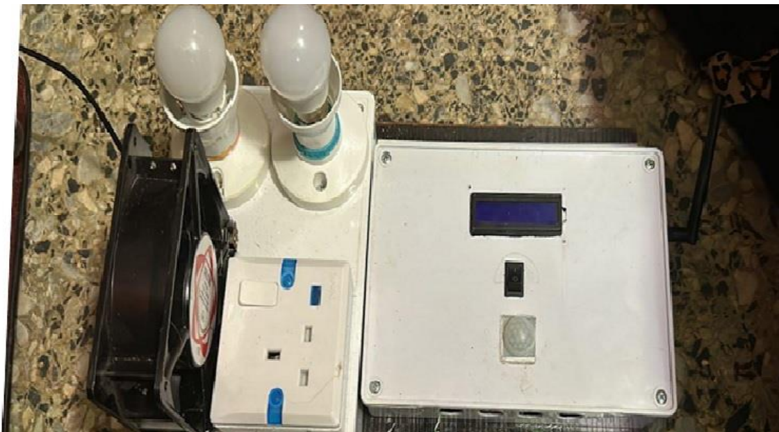
Figure 3: Completed design of the smart home automation system in OFF state
