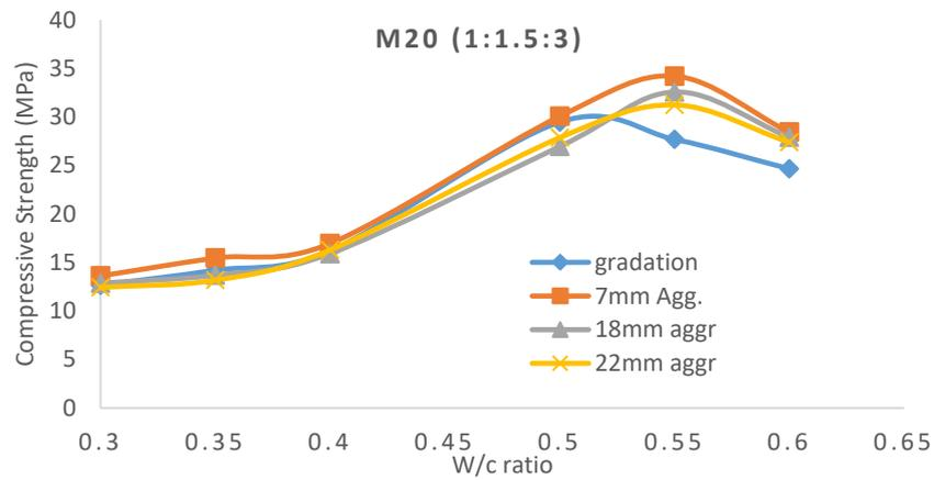
**Figure 2:** Strength variation due to aggregate sizes (M20)
