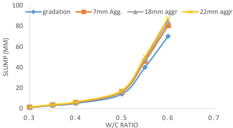
**Figure 6:** Workability variation due to aggregate sizes (M15)
