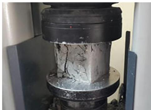
Figure 1: Compressive test
