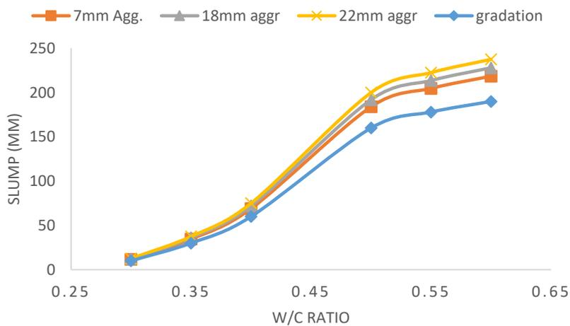
**Figure 5:** Workability variation due to aggregate sizes (M20)
