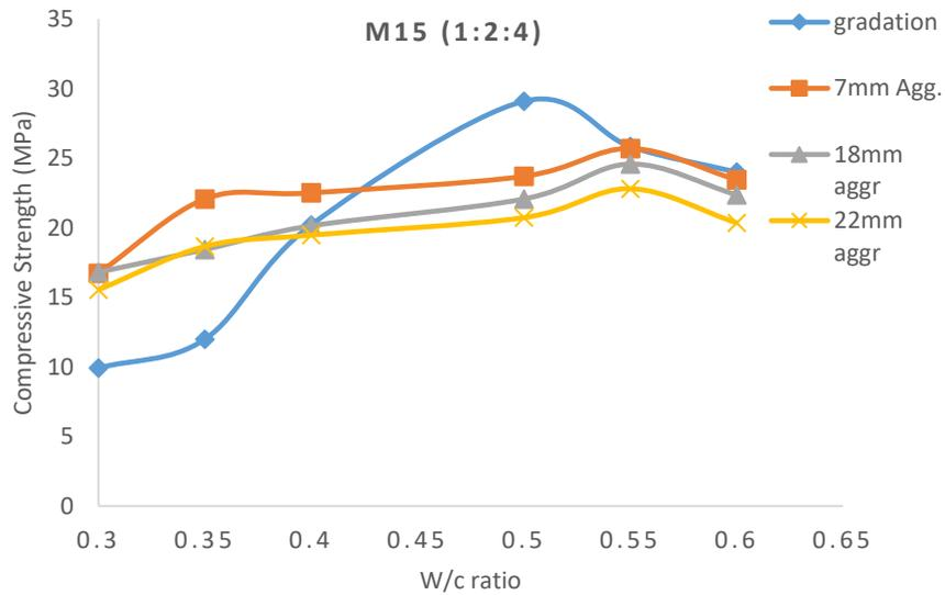
**Figure 3:** Strength variation due to aggregate sizes (M15)
