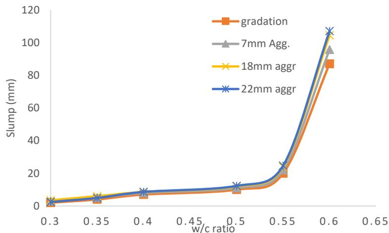
**Figure 7:** Workability variation due to aggregate sizes (M10)
