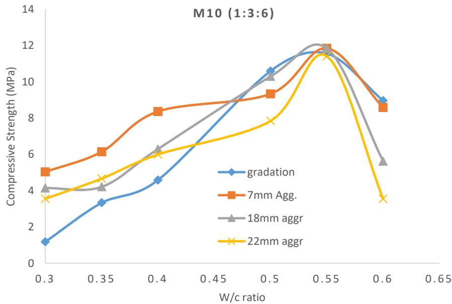
**Figure 4: Strength variation due to aggregate sizes (M10)**
