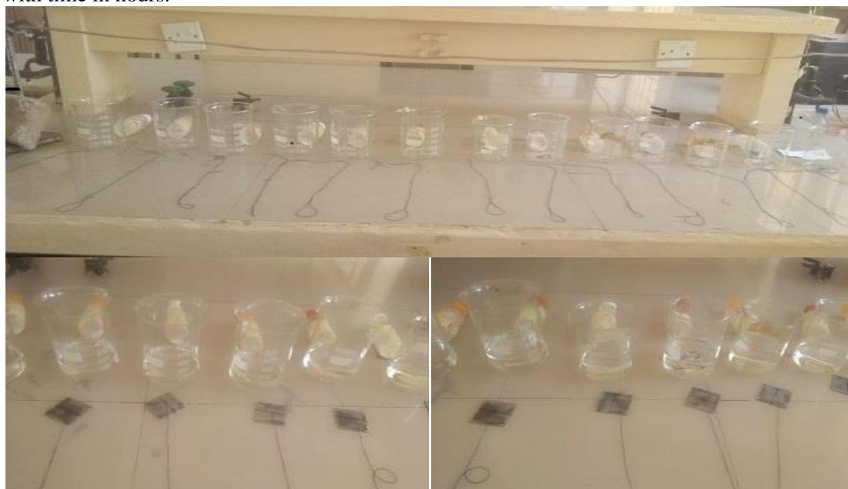
Figure 3: Set up for corrosion Inhibition
