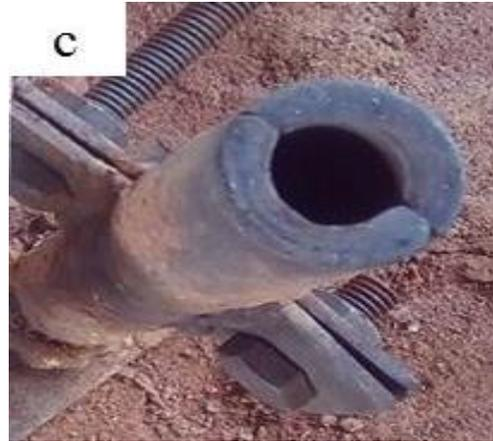
(c) Fabricated permanent mould
