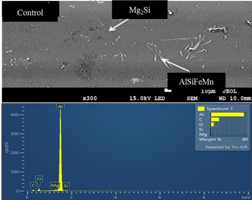
Figure 4. SEM-EDX micrograph of Al 6061 alloy as-cast
