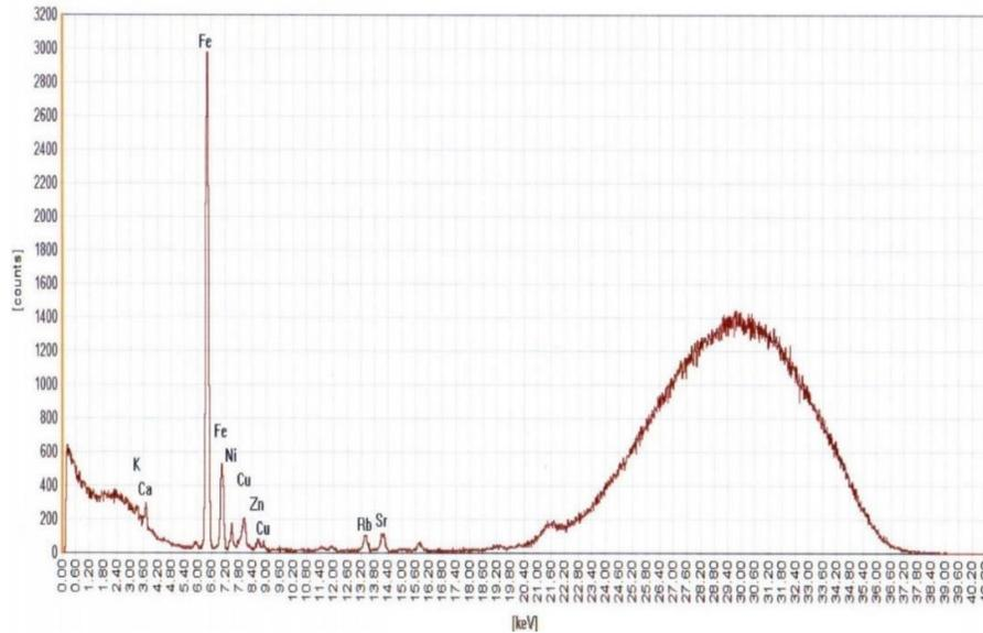
**Figure 3. XRF spectra showing the elemental constituent of the palm kernel shell ash (PKSA) particles.**
