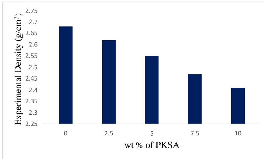
**Figure 1. Experimental density variation with wt % PKSA composites produced**
