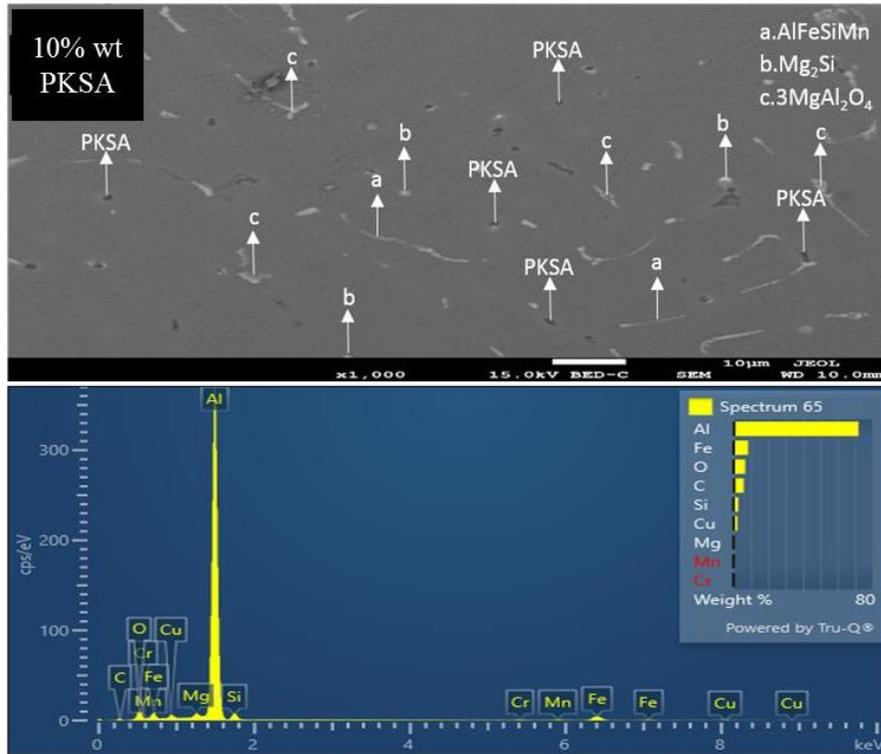
Figure 5. SEM-EDX micrograph of Al 6061 + 10%PKSA
