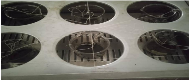
Figure 2. Experimental set-up of the measurements of weight loss in water bath
