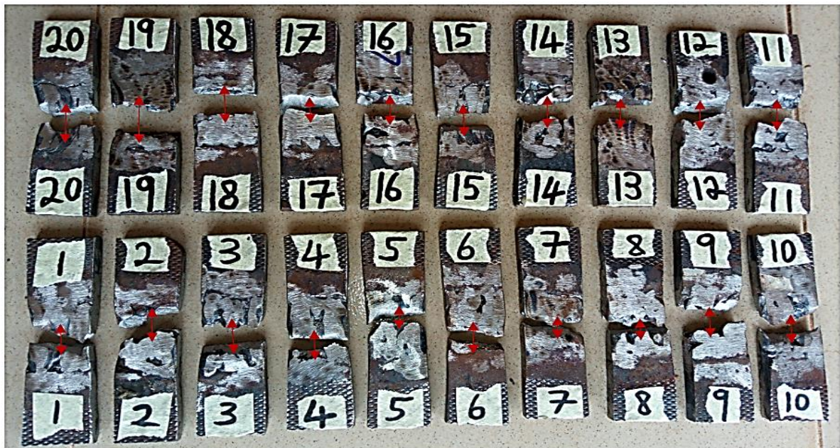
Figure 3. Test samples that have undergone tensile test from INSTRON tensile test machine
