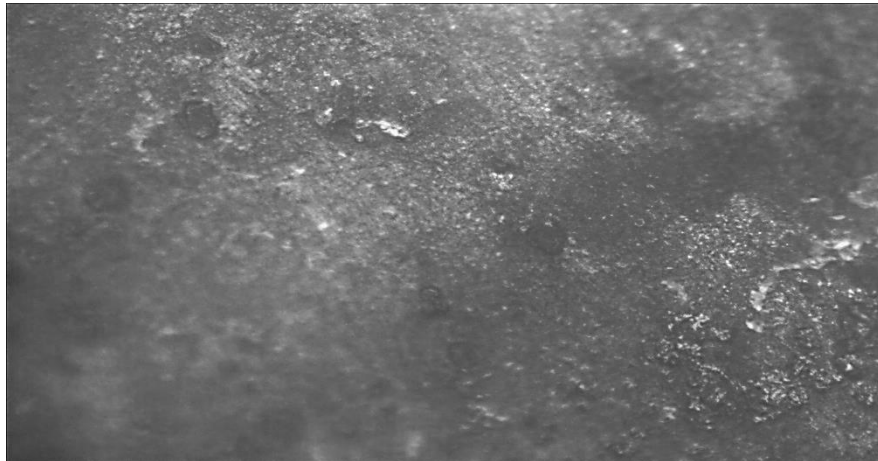
Plate 4.2c Micrograph of Tensile Test Specimen of BM for Low Heat Input (100A) at 200X
