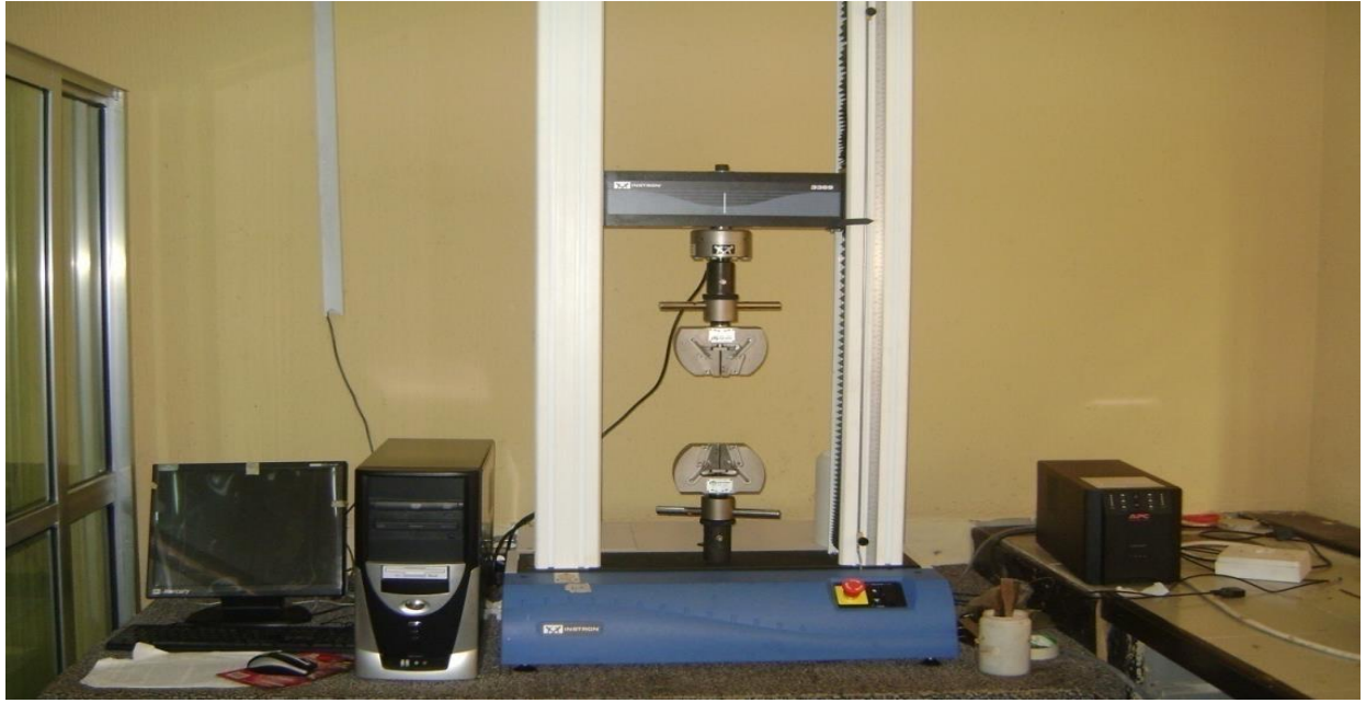
Computerized Instron Electromagnetic Tensile testing Machine (Model 3369): Source: UNN Department of Metallurgical and Materials Engineering
