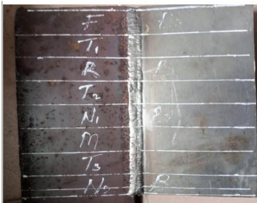
Figure 1. GTA welded AISI 316L ASS plate
