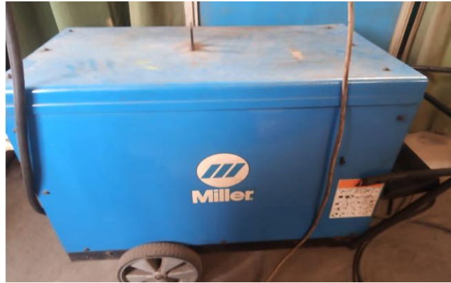
Figure 2. Gas tungsten arc welding machine
