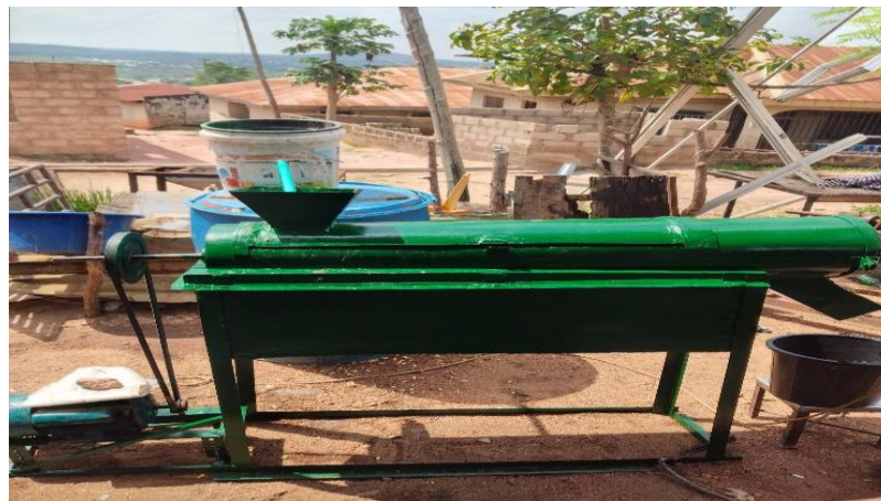
Figure 2: Pictorial view of the melon seed washing machine
