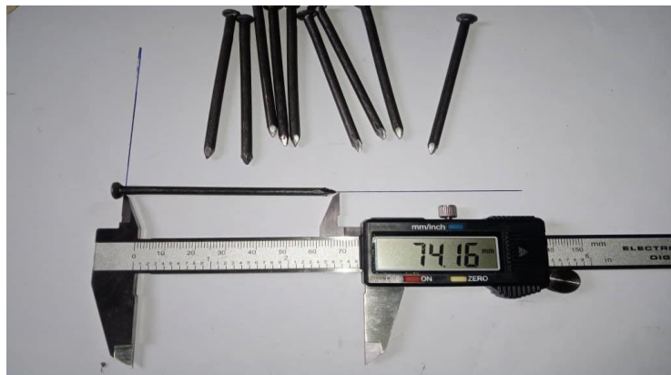
Figure 1. Vernier caliper reading of Nail Length (74.16mm)
