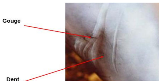
Figure 1. Pictorial presentation of the combined dent & gouge defect [3]
